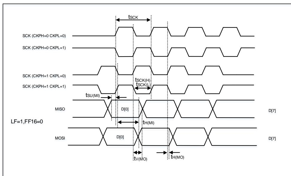
**Figure 4-9. SPI timing diagram - slave mode**
