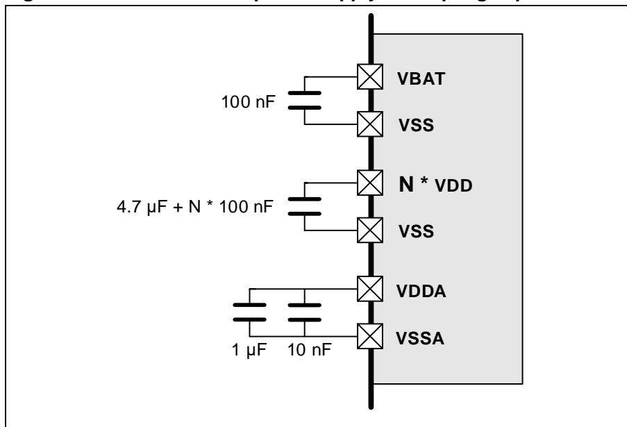
(1) All decoupling capacitors need to be as close as possible to the pins on the PCB board. More details refer to **AN057 GD32F3x0 Hardware Development Guide**.
