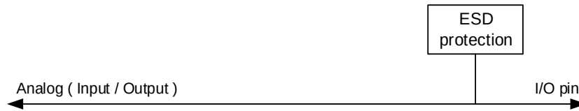
Figure 8-4. Basic structure of Analog configuration
