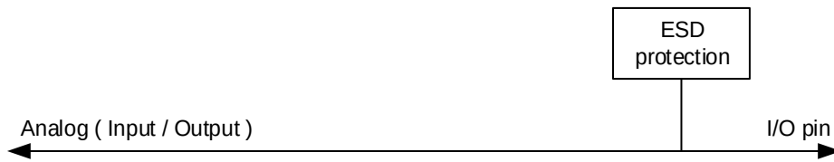
Figure 8-4. Basic structure of Analog configuration
