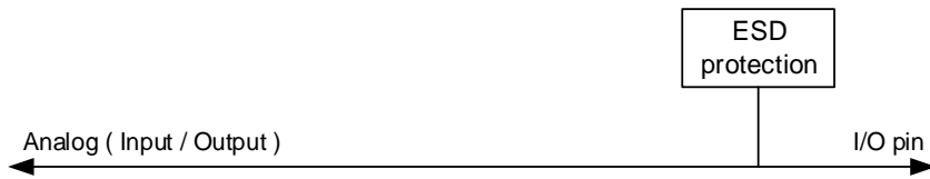
Figure 8-4. Basic structure of Analog configuration
