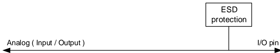
Figure 8-4. Basic structure of Analog configuration
