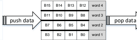
Figure 10-5. Data packing/unpacking when PWIDTH = '01'
