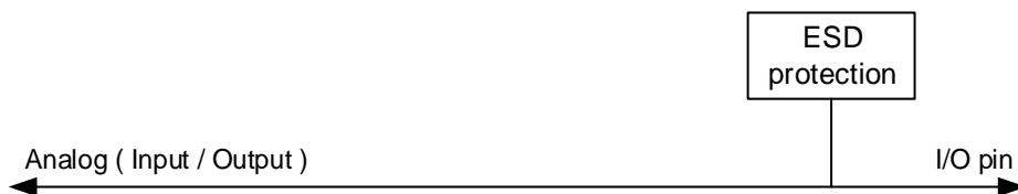
Figure 7-4. Basic structure of Analog configuration
