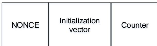
Figure 20-12. Counter block structure
