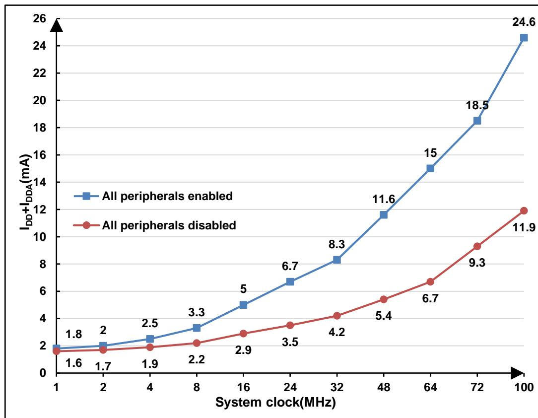
Figure 4-3. Typical supply current consumption in Sleep mode
