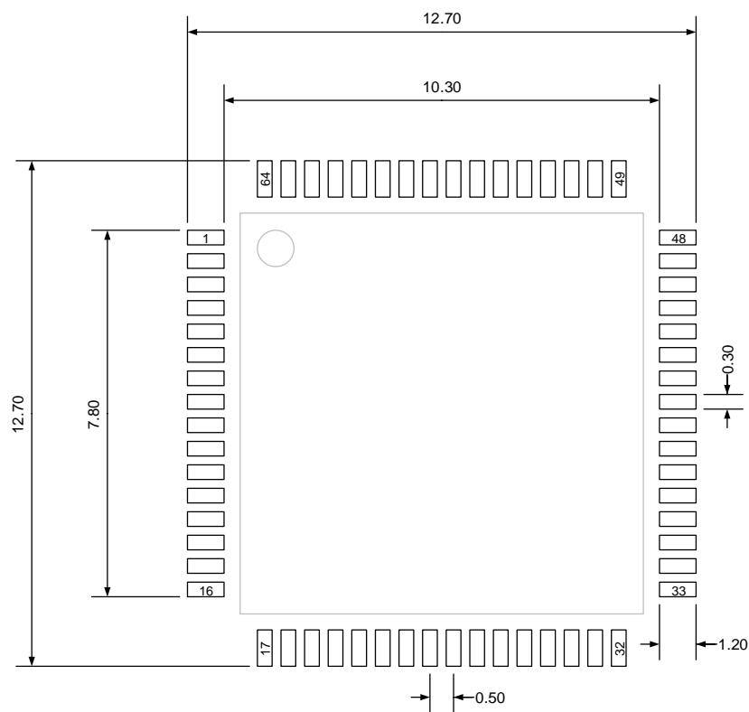
(Original dimensions are in millimeters)
