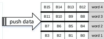
Figure 16-6. Data packing/unpacking when PWIDTH = '10'
