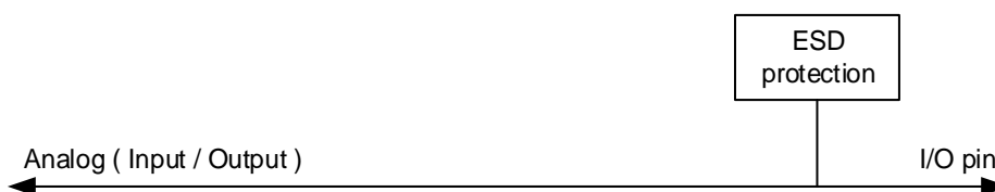
Figure 8-4. Basic structure of Analog configuration
