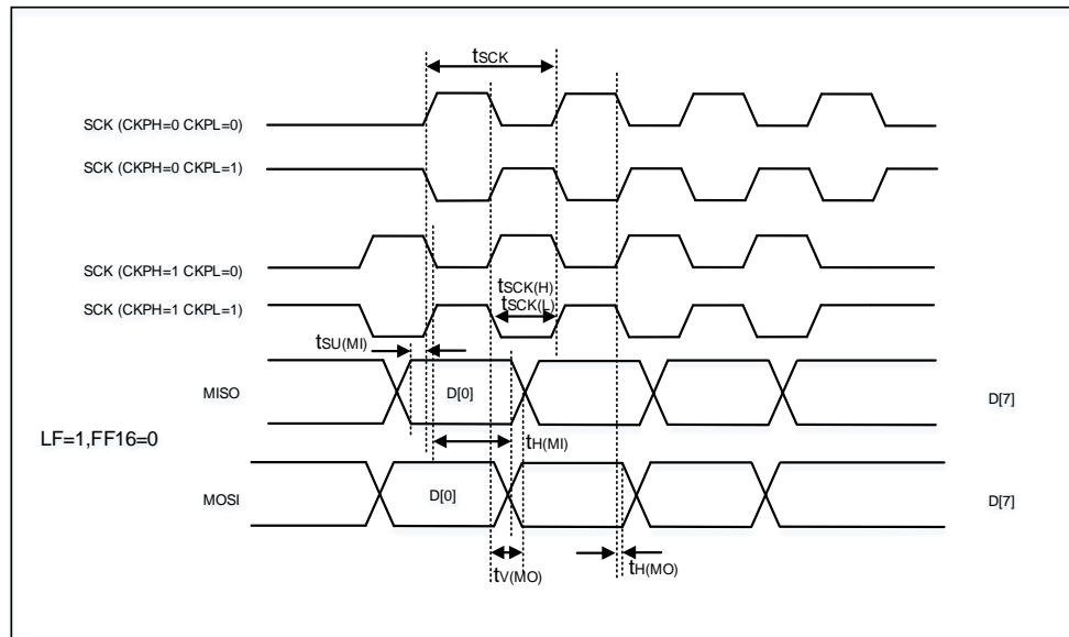
**Figure 4-5. SPI timing diagram - slave mode**
