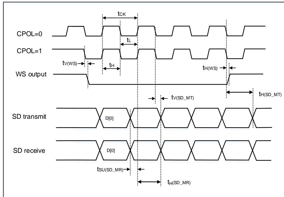
**Figure 4-7. I2S timing diagram - slave mode**
