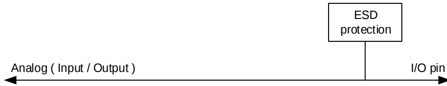
Figure 8-4. Basic structure of Analog configuration
