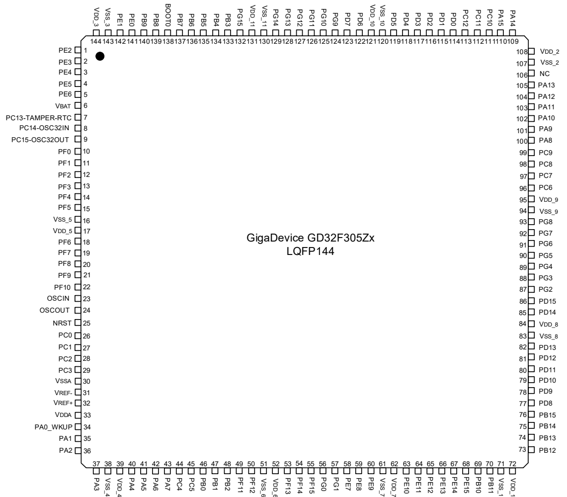
Figure 2-2. GD32F305Zx LQFP144 pinouts
