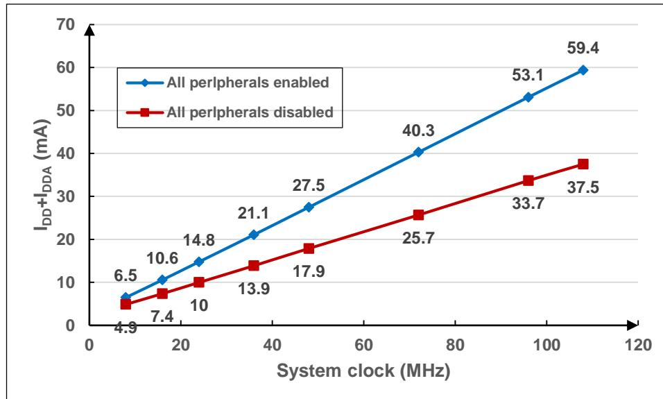
Figure 4-3. Typical supply current consumption in Sleep mode
