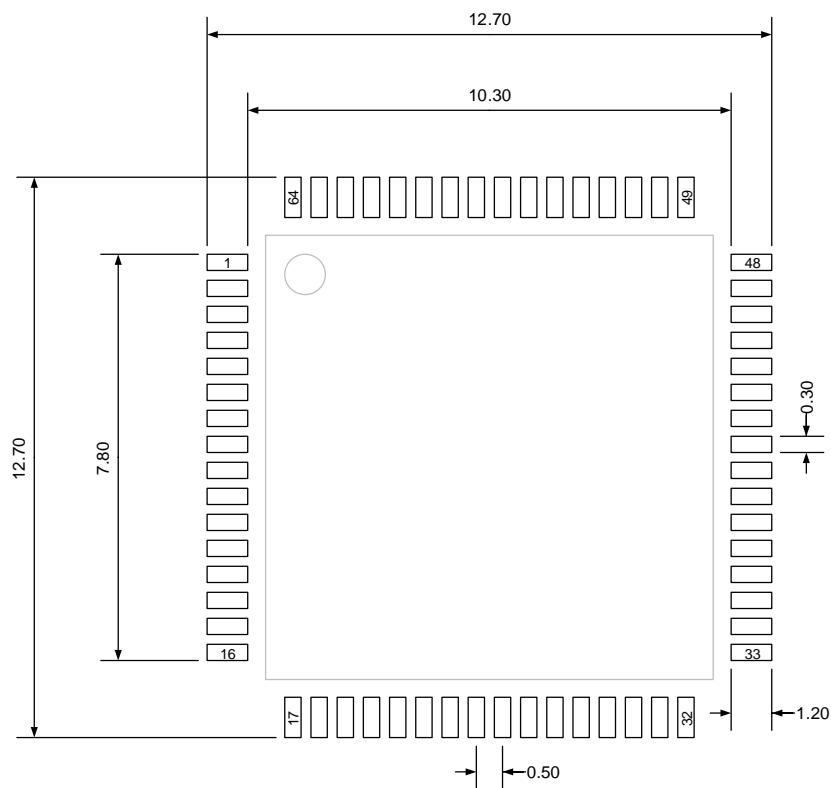
(Original dimensions are in millimeters)
