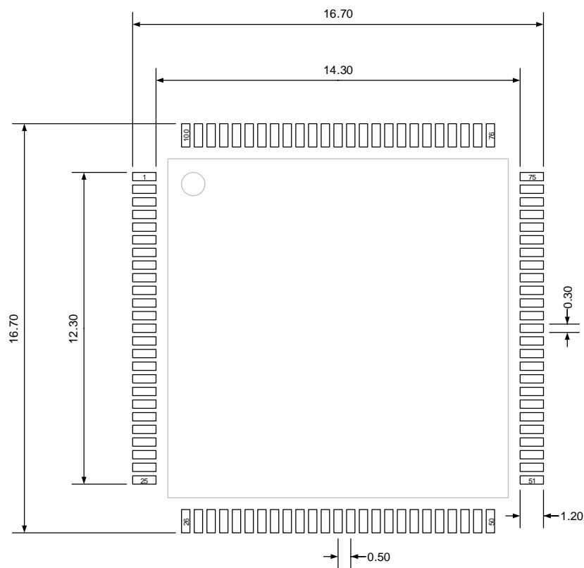
(Original dimensions are in millimeters)
