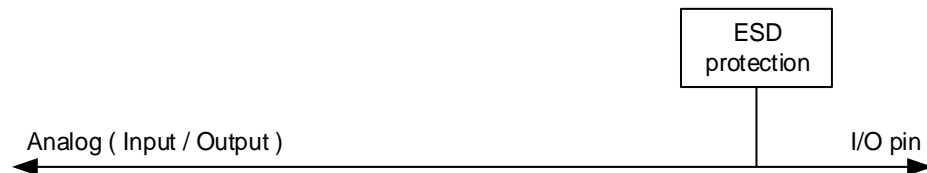
Figure 7-4. Basic structure of Analog configuration
