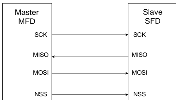
Figure 19-5. A typical simplex connection (Master: Receive, Slave: Transmit)
