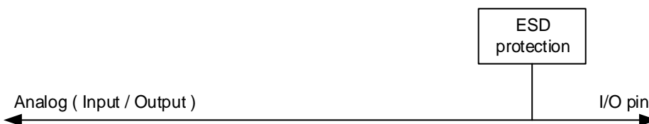
Figure 8-4. Basic structure of Analog configuration
