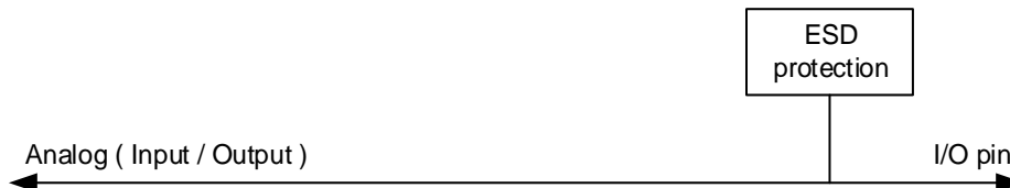
Figure 6-4. Basic structure of Analog configuration
