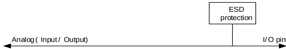
Figure 9-4. Basic structure of Analog configuration
