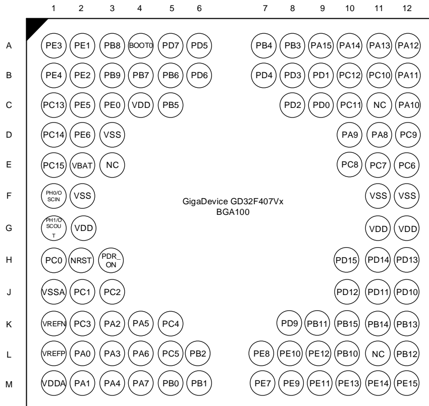
Figure 2-3. GD32F407Vx BGA100 pinouts
