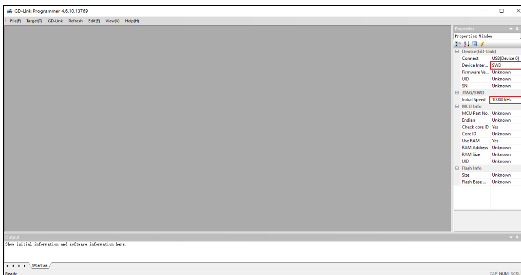
Figure 3-16. GD-Link programmer programming options configuration
