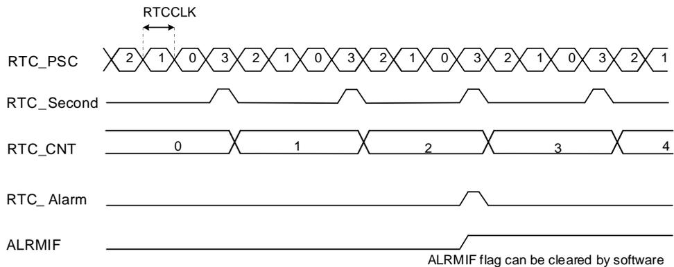
图 17-3. RTC 秒信号及溢出信号的波形(RTC\_PSC = 3)
