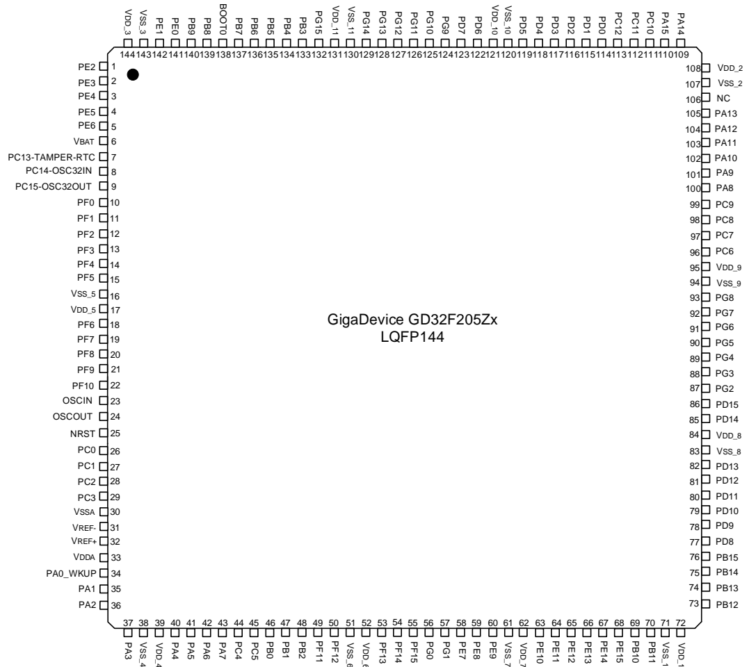
Figure 2-2. GD32F205Zx LQFP144 pinouts
